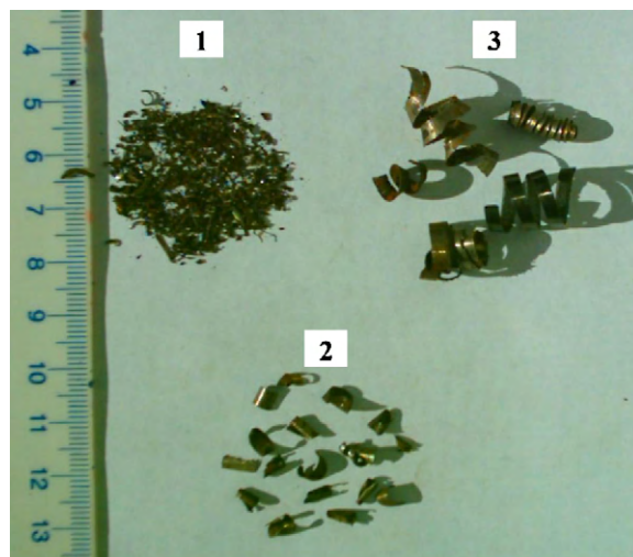
Fig. 1. Scrap iron used for Cr(VI) reduction: (1) powder; (2) shavings; (3) spiral fibers.
